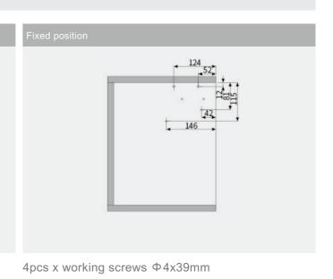
4 pcs x woodworking screws (Φ4x16mm) Use for fixing the aluminum panel 53+woodworking screws 12.5+T=Total length
